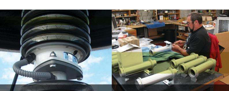
approach hazardous. The usual system of navigation in such places, which involved lining up two lights, was impossible because a cliff was in the way. So Norman Rumsey, head of optics in the physics and engineering laboratory of the old Department of Scientific and Industrial Research, devised a "sector light" — a single light that shows a different colour when viewed from different angles.
